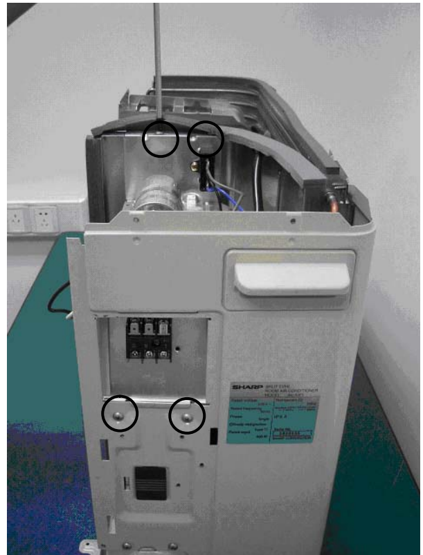
10) Loose 4 screws fixing the control box.
