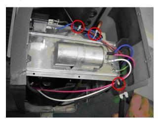
7) Remove 2 terminals. (connecting with fan condenser)
