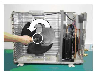
2) Loose 4 screws fixing fan motor.
