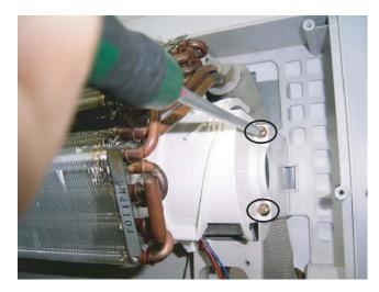
30)By holding up the left side of evaporator,take out fan motor with cover.
