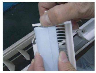
26)Remove the screw fixing cross flow fan.
