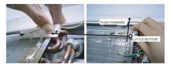
17)Remove 3 screws fixing the control box.
