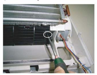
27)Remove 2 screws fixing the evaporator by the left side.
