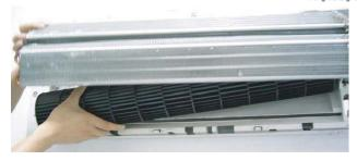
29)Remove 4 screws fixing motor cover.
