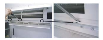
7) Remove 4 screws fixing the front panel.
