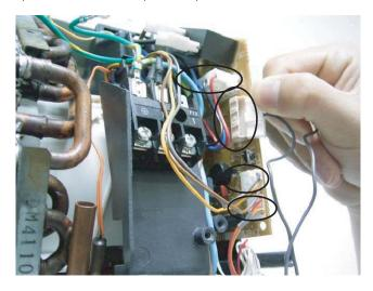
16)Remove the thermistor holder from the evaporator, push up the little button and then draw out.
