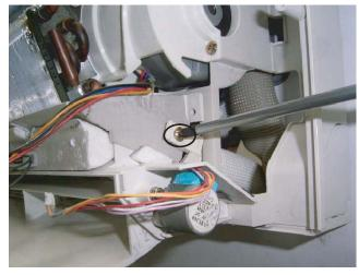
21)Release 4 hooks fixing drain pan.
