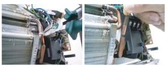
14)Cut the 2 bands fixing the wires.
