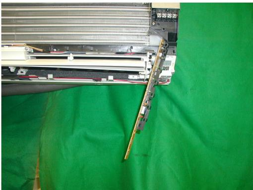
17) Remove a screw fixing the display guide.
