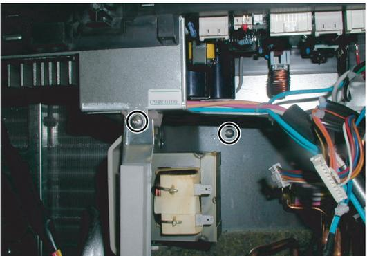
12)A bulkhead plate fixed 2 screws is removed.
