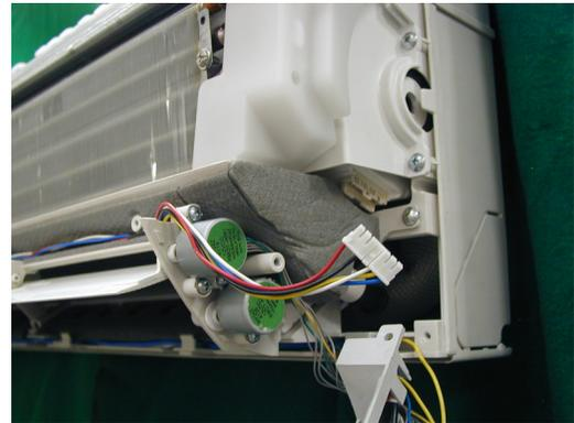
26) Remove 2 screws fixing the holder.
