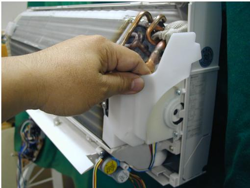
30) Remove the screw fixing the evaporator.
