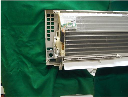
29) Remove the drain guide.
