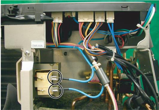
11)A control box BOX fixed 2 screws is removed.
