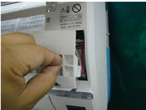
4) Remove the unit-to-unit wiring from the terminal board(4).
