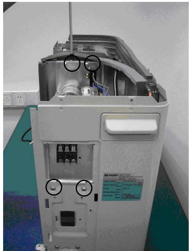
10) Loose 4 screws fixing the control box.
