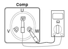
Disconnect the electrical connections to the compressor and check the resistance of the compressor windings, measure from U to V, V to W and W to U the values should be between 0.25 and 5 Ohms each.
