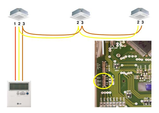
Next check the switch in the back of the remote controller, it has to be set to Group or GR1 for group control, the Factory setting is Single or SG, after setting the switch reset the power for 2 minutes. If the fault does not clear, check the Voltage of the remote controller cable.
