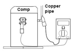
The next test is to measure the resistance of the compressor windings to earth.
